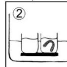
Clean pressure objects in a separate container with fresh SHERAultra-p for a maximum of three minutes in an ultrasonic bath (total time not more than 10 minutes!).
