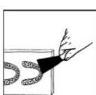
Remove finished printed works and any polymerised residues from the building platform by using a spatula.
