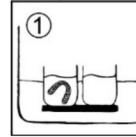
Clean pressure objects in a separate container with SHERAultra-p for a maximum of three minutes in an ultrasonic bath.
